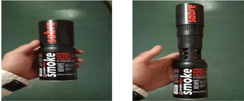
**Gambar 3. Smoke Detector Tester**
