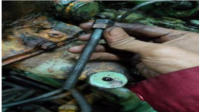
**Gambar 3.** Baut Pondasi *Intercooler* KM. JML ABADI
