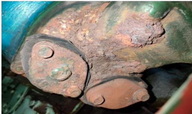
**Gambar 1.** Cover In *Intercooler* Kapal KM. JML ABADI
